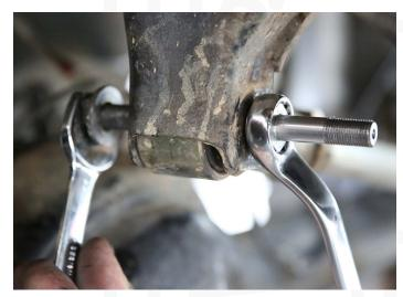
3. Loosen the pinch bolt on the Fox damper until the mount is free to rotate.
