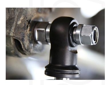
5. Orient the reservoir upward and loosely mount the other end to the draglink using the supplied collars that were test fitted in step one.
