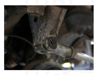
2. Install the supplied stud as per image re using the standard nut from original bolt, note stud is to face forward.
